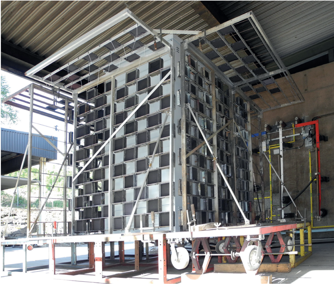
Figure 7, ABB SafeRing/SafePlus 36 kV switchgear under internal arc testing
