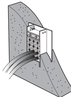
The B frame cast and sealed in concrete wall.
