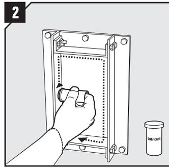
2 Lubricate the inside surfaces of the frame with Roxtec Lubricant, especially into the corners.
