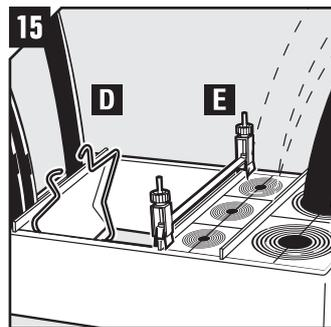
15 Stayplate clips (D) and stayplate clamps (E) can be used to simplify horizontal assembly.
