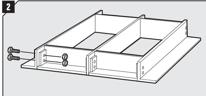
Assemble the frame parts by inserting all bolts and touch tight the nuts. When completed, tighten the nuts fully. The B frame can easily be assembled around already routed cables or pipes.
