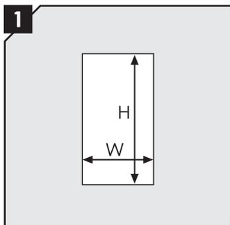
1 Mark a rectangular opening according to frame type (see table below).
