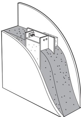
Before concrete is poured, the frame and casting mould are fixed in position with the frame flange inside the wall.
