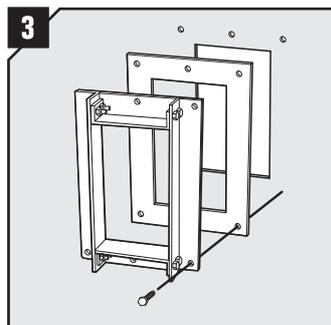
3 Attach the frame to the cabinet/wall using bolts and nuts. An optional rubber gasket can be placed between frame and cabinet/wall.
