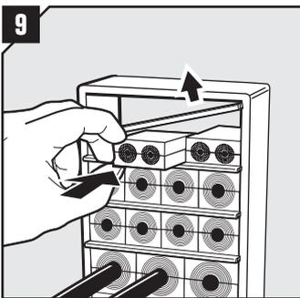
9 Separate the two stayplates and insert the final row of modules between the stayplates.
