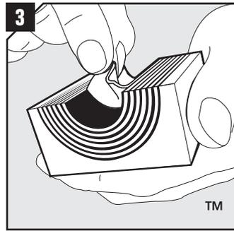
3 Adapt modules, which are to hold cables or pipes, by peeling off layers until you reach the gap seen in pic. 4. The halves may not differ by more than one layer.
