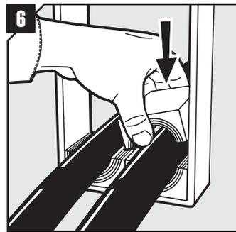
6 Insert the modules according to your installation plan (transit plan). It is recommended to seal cables/pipes at the bottom of the frame and put spare modules on top.
