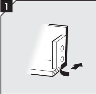
Remove the protective foil from the sealing strip on all short sides.
