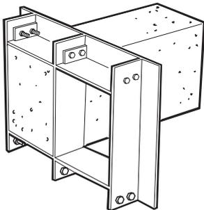
For correct casting of frames into concrete walls, casting moulds in cellular plastic are available.
