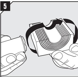
5 Lubricate all modules for the frame thoroughly, both the inside and the outside surfaces.
