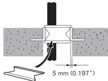
The size of the opening in the structure must be 5 mm (0.197") wider than the inside dimensions of the frame on all sides. The stayplates need this space to be able to move inside the frame during installation and compression.
