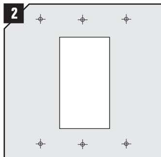
2 Use the frame as template for the drilling of the screw holes. Hole in flange  $\varnothing = 9 \text{ mm}$  (0.354").
