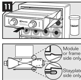
11 Lubricate all sides of the wedge sparsely, except front and back. Please read the markings on the wedge and turn it correctly before inserting it in the top of the frame (standard position). Face with "Stayplate this side" must always face a stayplate.
