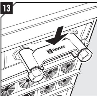
13 Attach the Wedge Clip to the wedge bolts to check that the wedge is properly tightened.
