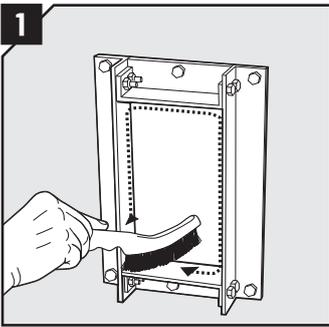
1 Make sure that the inside surfaces of the frame are free from dirt or dust.
