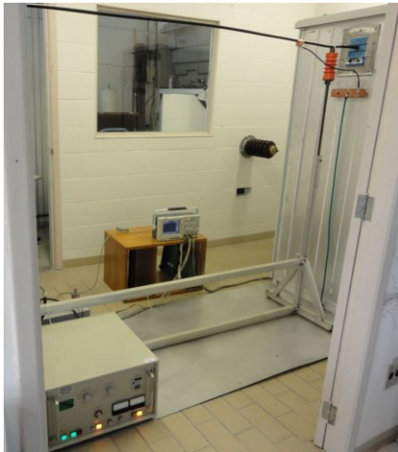
Fig. 4. General view of the test setup showing the current surge generator, coaxial cable, shielded cabinet, ground plane and digital oscilloscope; The shown configuration corresponds to Case 1, Fig. 2(b).
