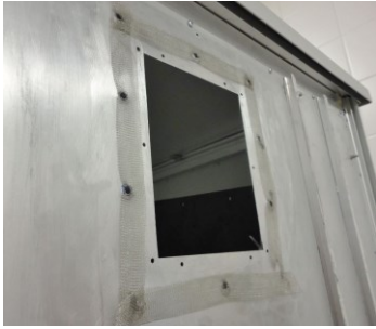
(a) Feed-through window with braided tape; 0.15 x 0.18 m opening.
