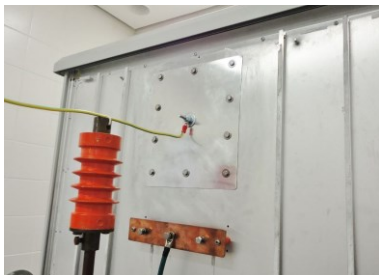
(e) Case 4: Aluminum plate and 6 mm 2 cable.
