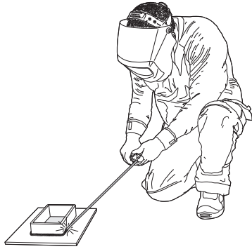
Horizontal MMA welding
