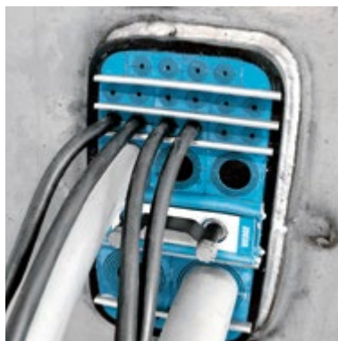
Stress exposed bulkhead. Roxtec SRC has rounded corners to reduce stress in bulkheads around cable penetrations. Available in different versions and dimensions.
