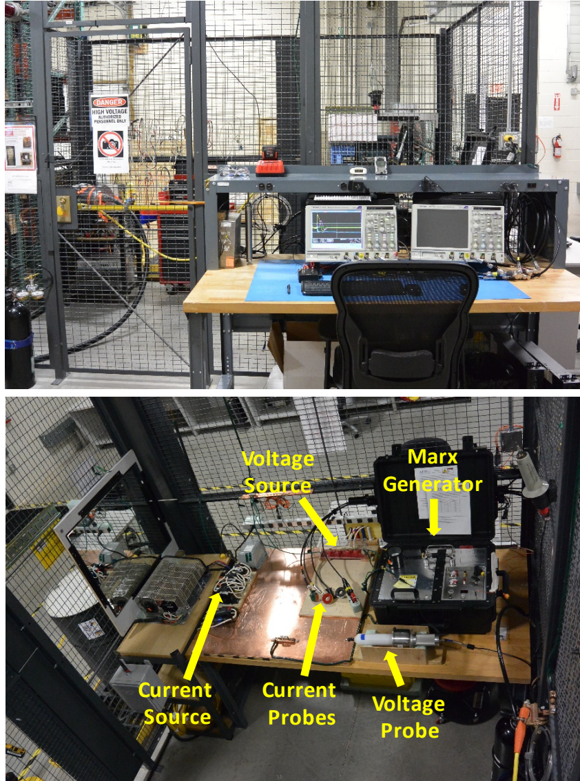
Figure 3-13 Illustration of EPRI's direct injection test based on MIL-STD-188-125-1 Note: DUT is not shown
